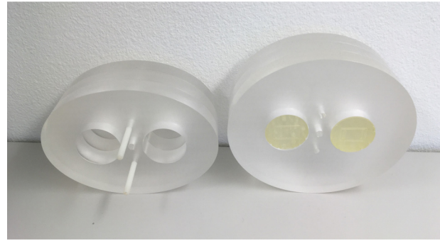
Figure 1. Two body phantoms of different size. The left phantom has an effective diameter of 27 cm and the right one an effective diameter of 32 cm. Two DDC modules are installed in the right phantom, the corresponding holes in the left phantom are unpopulated.
