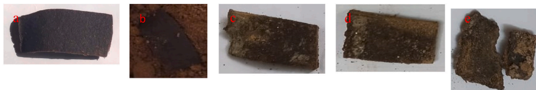
Fig. 2. Soil biodegradability of the sample S1 after (a) 0 days (5 gm), (b) 7 days (14), (c) 15 days (20), (d) 21 days (40), (e) 30 days (60).
