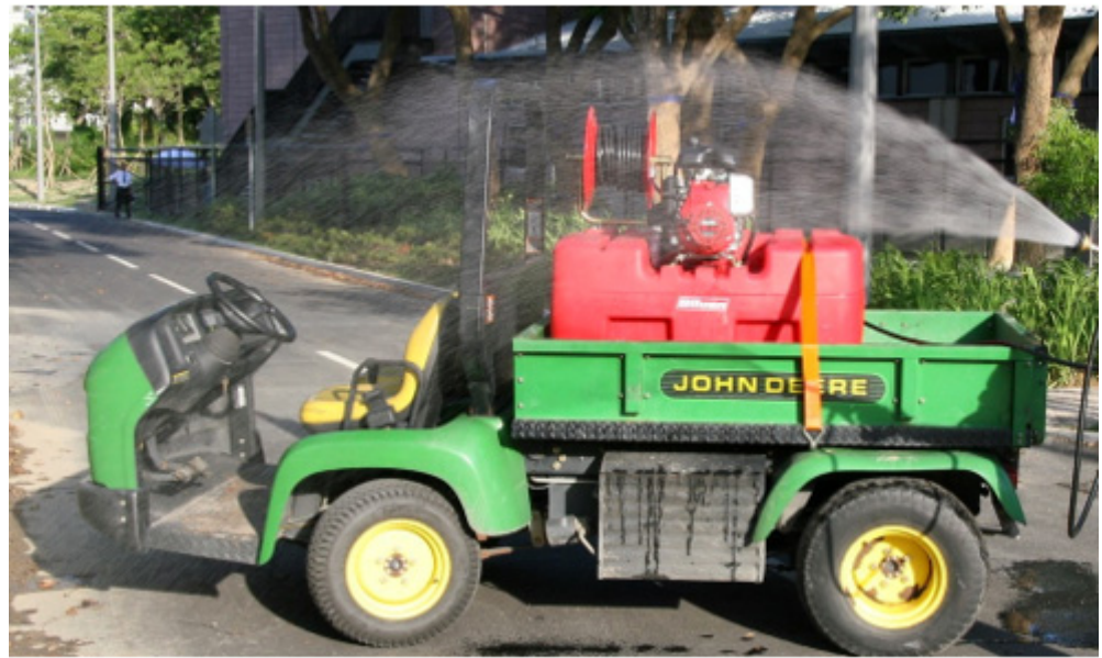
Figure 22. A cold-water spray unit in use at the Hong Kong Jockey Club.
