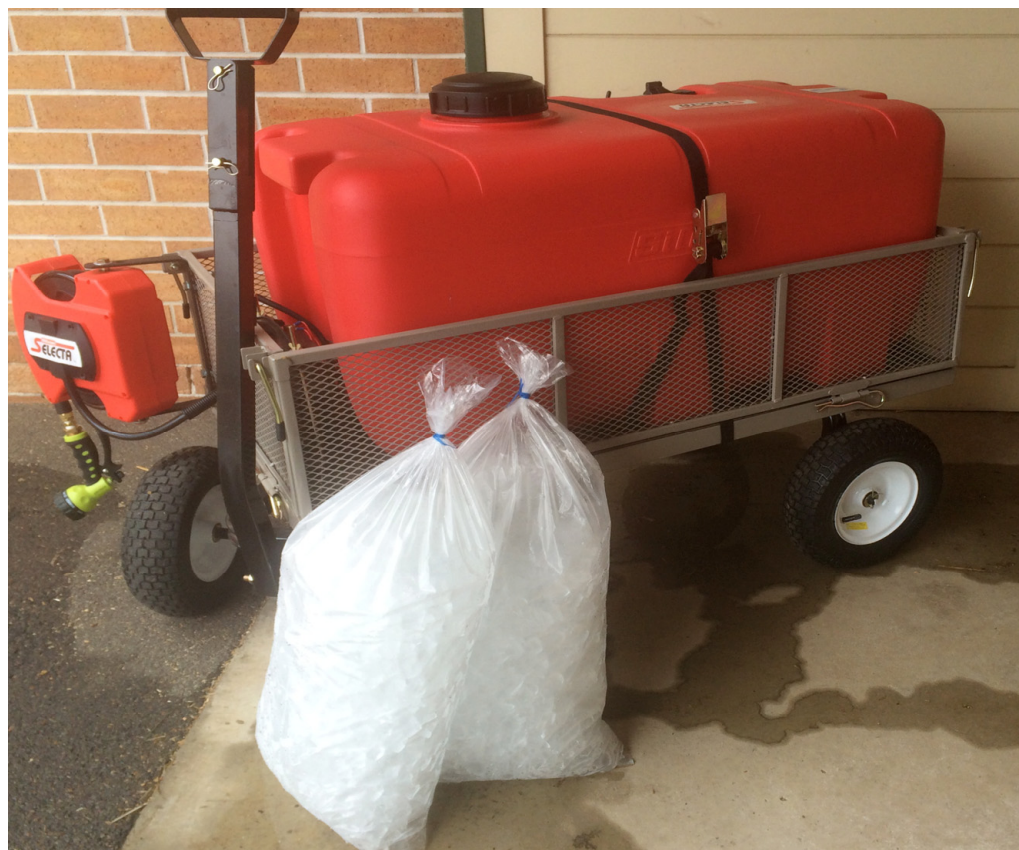
Figure 21. A compact, mobile cooling device. The design could be improved by the inclusion of an insulating blanket to decrease ice loss in the hot summer months and a wider filler neck to admit solid ice more easily.
