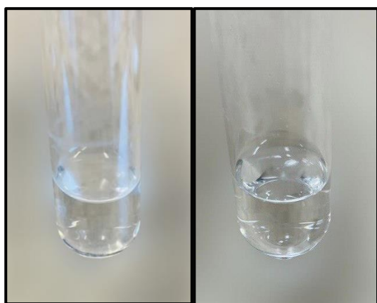
Fig. 4. Images of samples of the solubility test of the model drug dextromethorphan in the laboratory prepared lysosomal fluid (SLYF) where it fully dissolved (right) and in the commercial artificial counterpart where the fluid was turbid with a precipitate formed (left).
