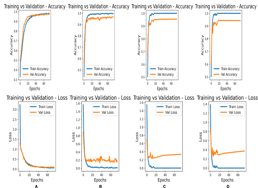
Figure 4. Accuracy and Loss curves for training and validation of the second data-fold for various CNN architectures. (A) Complete Fet-Net architecture. (B) No dropout in the feature extraction component. (C) No dropout in the feature extraction component or classification component. (D) No dropout in the feature extraction component or classification component, and no hidden dense layer of 256 neurons.
