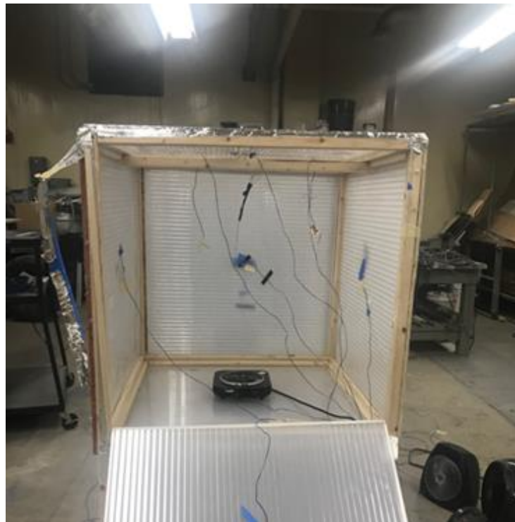
Figure 5. Aerogel box for experimental validation.
