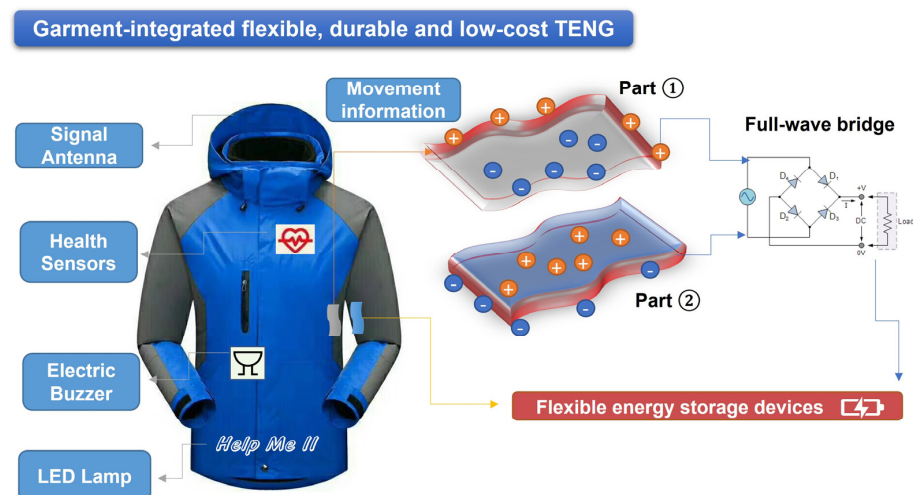
Figure 9. The potential applications of the flexible and robust G-TENG. To facilitate storage, a rectifier bridge can be added to the system to convert alternating current into direct current, and a flexible energy storage device can be used to collect the electrical energy harvested from everyday activities.
