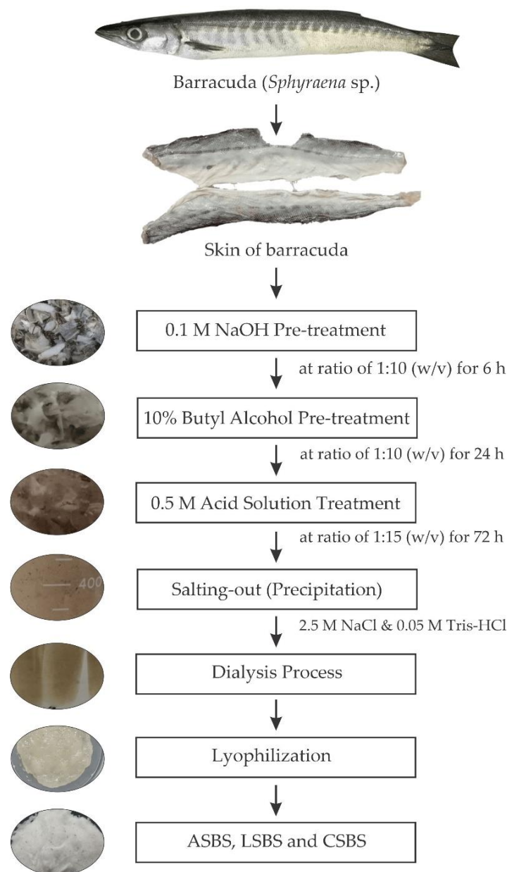
Figure 1. Flowchart of acid-solubilized barracuda skin collagen production. ASBS: acetic acid-solubilized barracuda skin collagen; LSBS: lactic acid-solubilized barracuda skin collagen; CSBS: citric acid-solubilized barracuda skin collagen.
