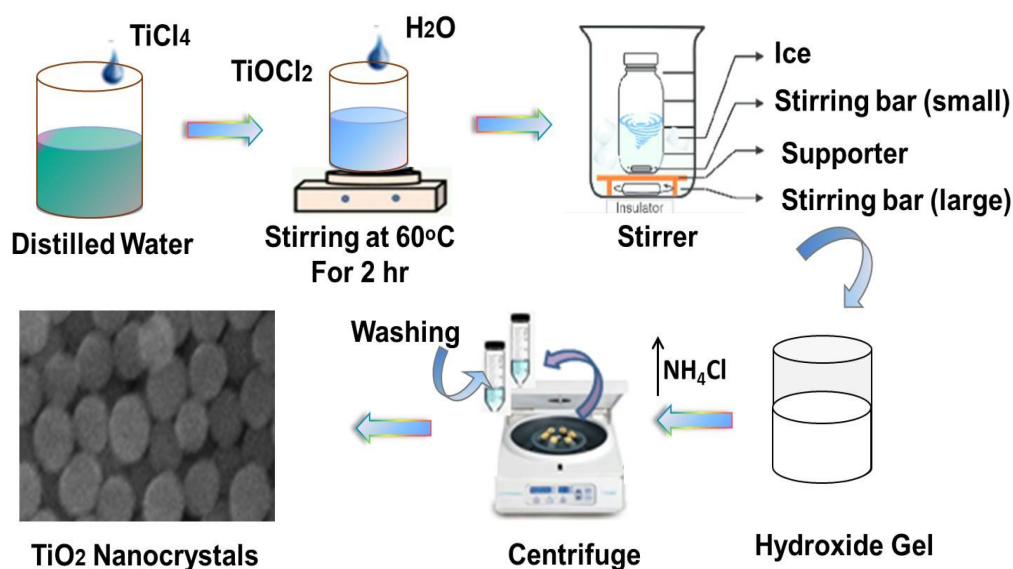
Figure 1. Schematic illustration of the TiO 2 nanoparticles synthesis process.
