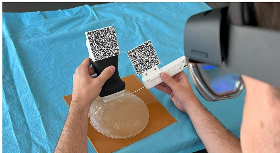
**Figure 8.** Third-person usability test view of a user performing the biopsy in a breast phantom.
