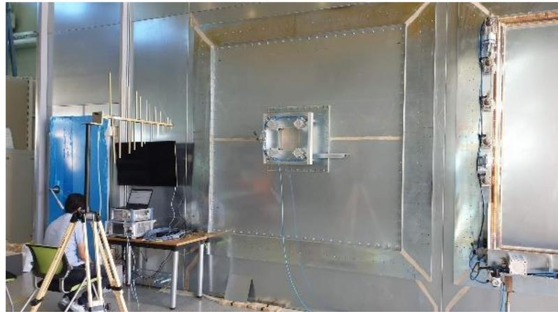
Figure 11. Shielding effectiveness measurement of concrete.
