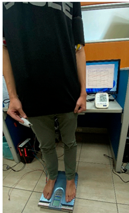
Figure 5. A photo from this experiment shows a subject standing on a commercial body weight-fat scale. The finger of right hand wears the PPG probe, a cuff is wrapped around the left arm, and two electrodes of the ECG are placed on the right and left arms.
