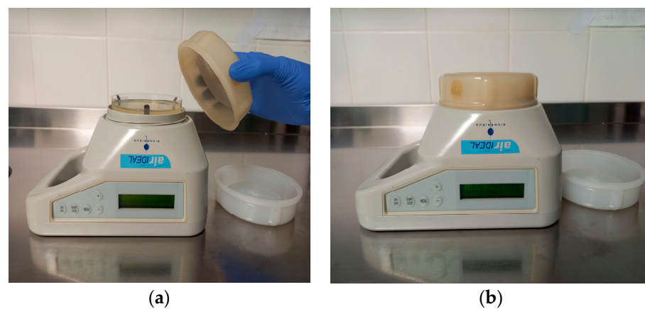
Figure 2. Air sampling with portable air sampler. (a) Preparing of air sampler for sampling procedure. Petri dish with Sabouraud medium is placed and covered with sterile sample grid. Time of duration and volume of air to be sampled is defined and visible on display. (b) Air sampling in process. Air containing spores is aspirated and inoculated through a sampling grid onto growth medium.
