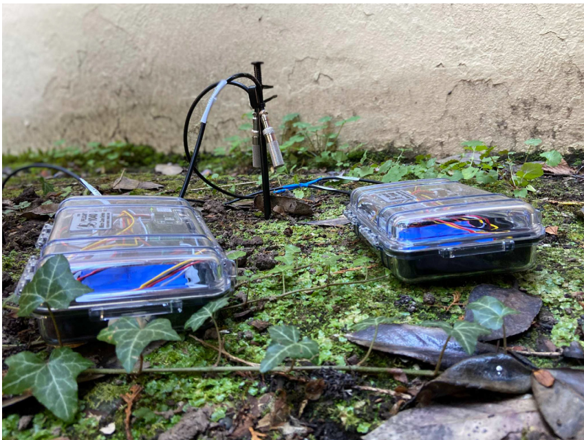
Fig. 17. SHT-30 sensors zip-tied to tent stake.
