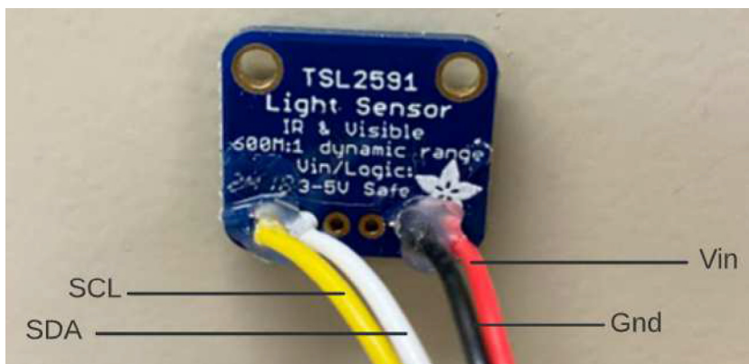
Fig. 14. TSL2591 with JST wires connected.
