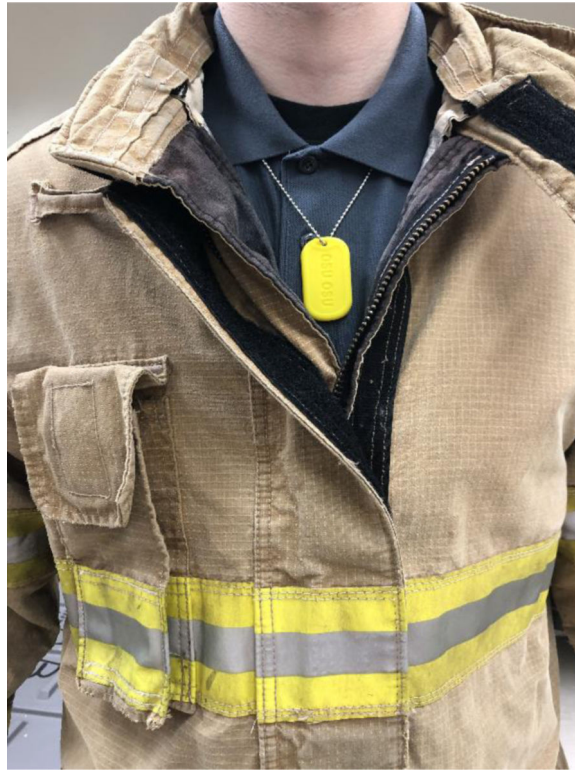
Figure 1. Silicone dog tags (shown in yellow) were worn around the neck underneath firefighting personal protective equipment.
