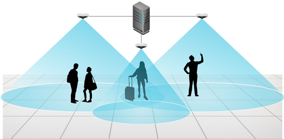
Fig. 3 Illustration of the considered scenario. Multiple omnidirectional cameras with a small overlap cover the monitored area. The cameras are connected to a central GPU-enabled server
