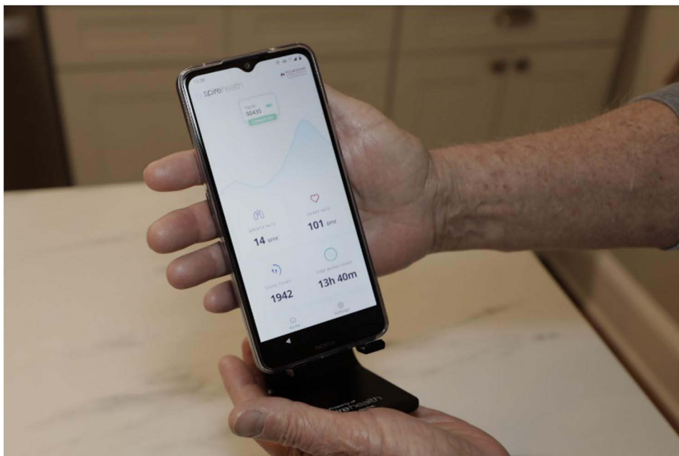
Figure 2 The hub passively captures sensor data and securely transmits it to the cloud. It provides limited feedback to patients.
