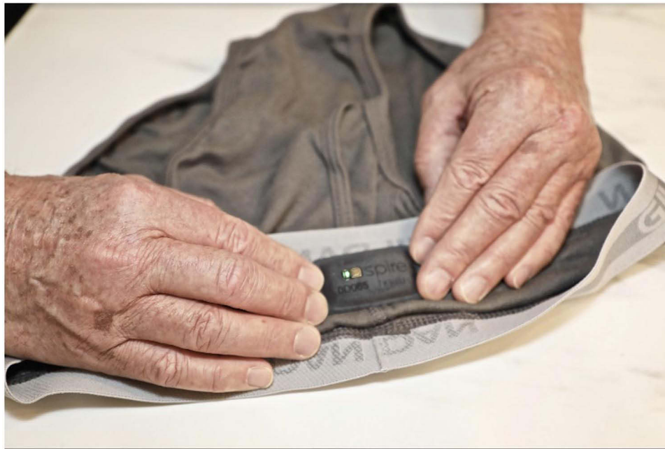
Figure 1 The sensors included in the RPM service are adhered to undergarments to address the burden involved in maintaining a clip-on or wrist-worn sensor, without requiring skin-adhesion.
