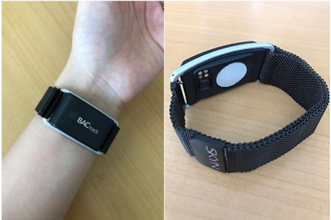
FIGURE 1. BACtrack Skyn. Views of the alcohol biosensor used in this study
