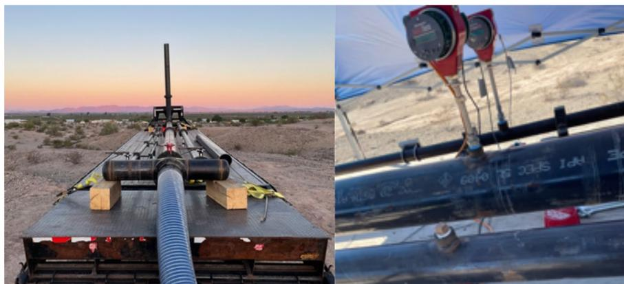
**Figure 5.** Metering and release trailer (left) has four pipes (0.5-in., 2-in., 4-in., and 8-in.), each leading to a distinct metering location allowing a different dynamic range of release volumes. The three larger pipes used a Quadra Therm 640i insertion meter (right), with upstream 8.5 m straight run of pipe to ensure sufficient flow stabilization for all pipes. The 0.5-in. pipe was not used in this study.
