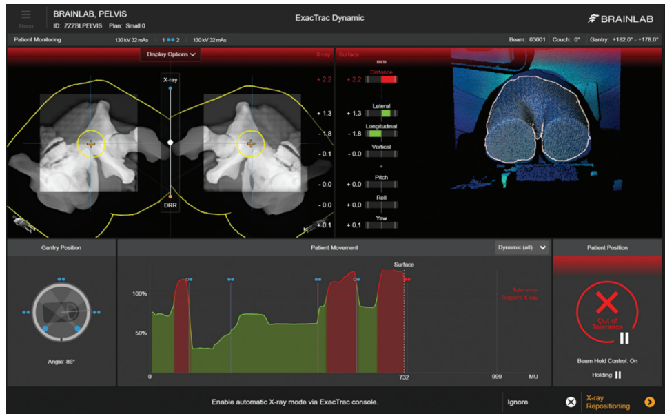
Figure 6: ExacTrac display while remotely moving the Brainlab pelvis phantom using the 2D motion platform
