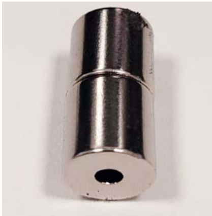
► Fig. 2 Custom-made magnetic neodymium rings.
