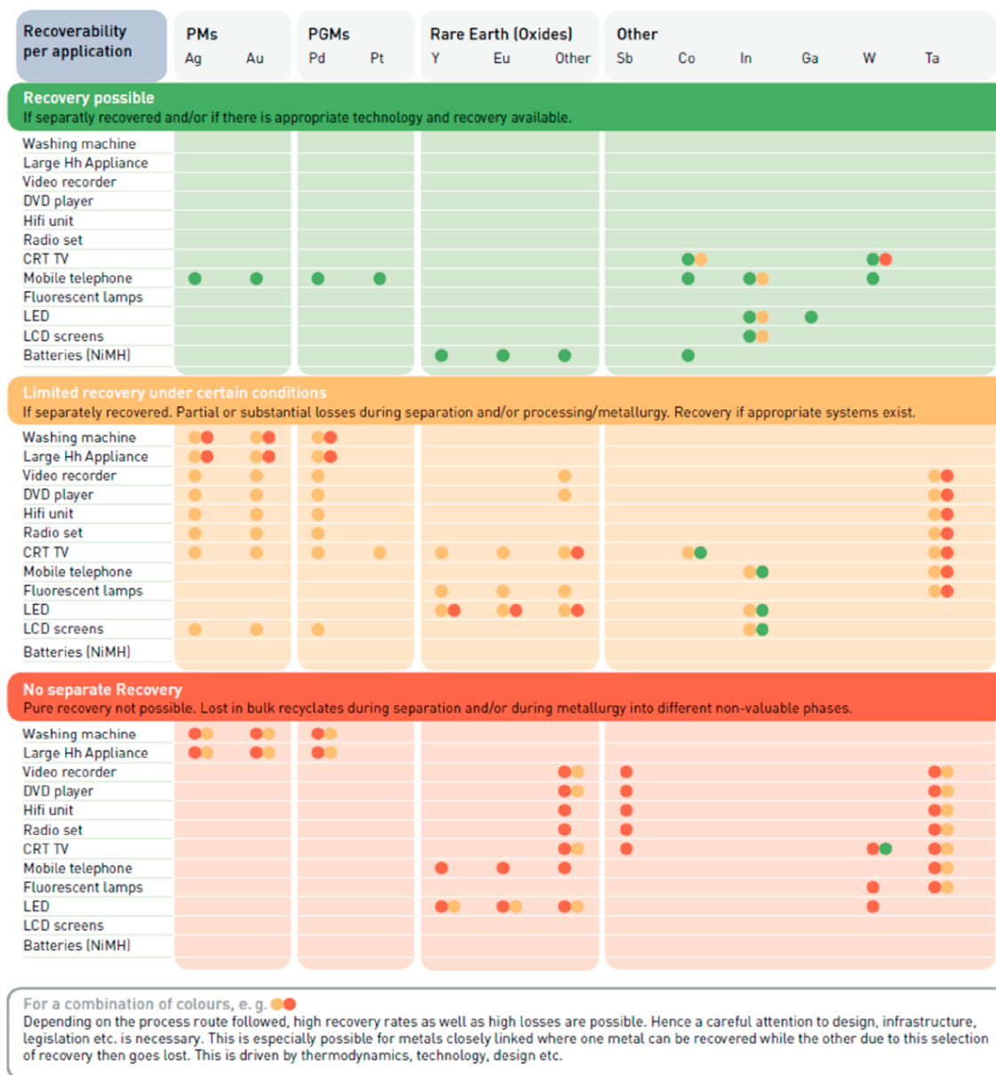
Figure 34. Metals that can be recycled from several types of products and metals that are hard to recover. 156 The figure is reproduced with permission from ref 156. Copyright 2013, UN Environment Programme UNEP.
