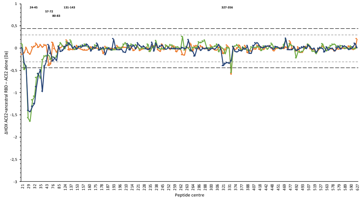
Supplementary Fig 27. Difference plot illustrating the difference in HDX between ACE2 in complex with the isolated ancestral RBD and ACE2 alone (orange line indicates: 20 s on ice, green line: 10 min at 23 °C, dark blue line: 360 min at 28 °C). Peptide segments of interest are highlighted. The peptides are arranged according to their peptide centre residue. A dotted grey line indicates the 98% CI as a threshold for significance and a dotted black line the 99% CI as a threshold for significance.
