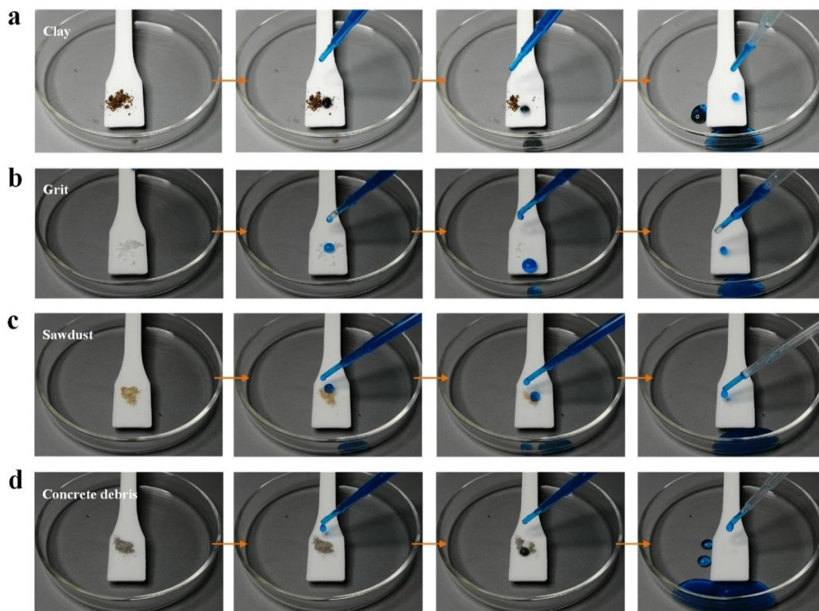
Figure S8. Self-cleaning of diverse dirt on the printed superhydrophobic surfaces. a) Clay, b) grit, c) sawdust and d) concrete debris were put onto the printed superhydrophobic surfaces. Several dyed water droplets were then spread onto the printed superhydrophobic surfaces to test the self-cleaning property. The printing parameters for these samples are 4 wt% HFS/PP weight ratio and a laser power density of 0.0725 \text{ J/mm}^2 .
