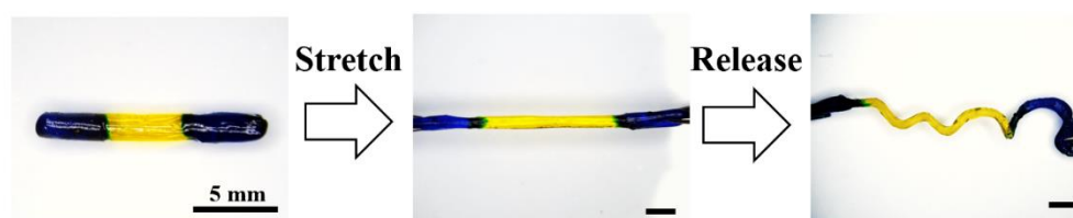
Fig. S6. The stretching process of the self-healed G3K/OHA hydrogels. After 20 min of healing, the reunited hydrogel cylinder was stretched up to 500% strain.
