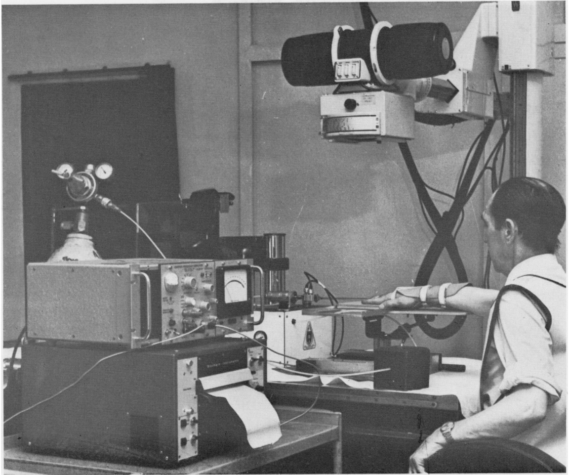
FIG. 1 A machine designed to 'crack' the metacarpophalangeal joints of human subjects.
