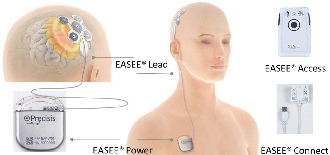
Figure 1 EASEE System elements
