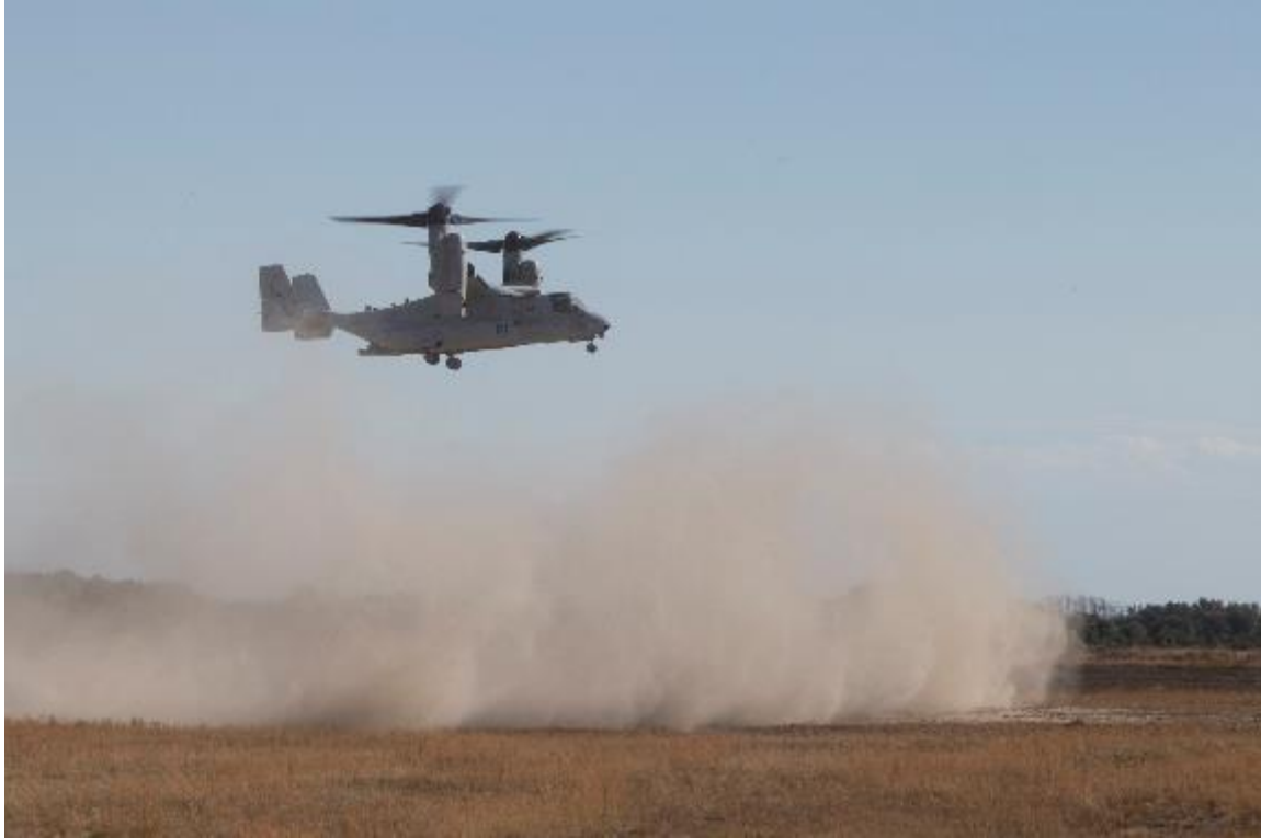
Figure S3. Although typical ‘brownout’ dust clouds generated by rotorcraft are only 2-3 rotor diameters across and form within one or two diameters of the ground, occasionally separated clouds can be seen. This one, with geometry very similar to that observed for Ingenuity at Jezero is a MV-22 Osprey tilt-rotor aircraft on exercises at Camp Lejeune. US DoD Photo 171130-M-CO135-095 by U.S. Marine Corps Pfc. Ginnie Lee.
