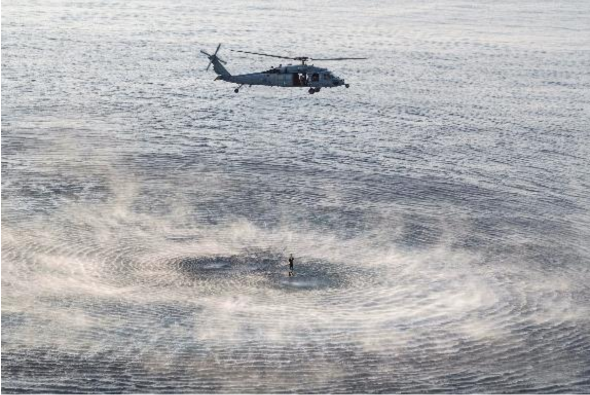
Figure S2. A Navy MH-60S Seahawk helicopter during anti-mine countermeasures training in the Gulf of Aden, 2019. The ripples and spray provide a graphic indication of the shear stress imparted by the downwash a couple of diameters below and beyond the rotor disk. U.S. Department of Defense Photo 190410-N-HX510-0179Y by Navy Seaman Jarrod A. Schad.
