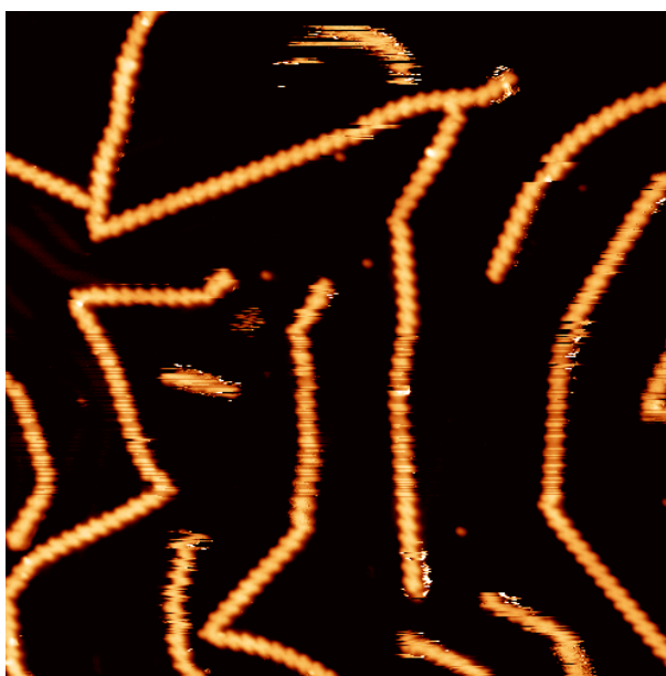
Figure S6 STM image confirming the selective formation of polymer 4 (composed of monomers having formed five-membered rings). STM parameters: (50 nm × 50 nm) I = 10 pA, V = 1.0 V, T = 78 K.
