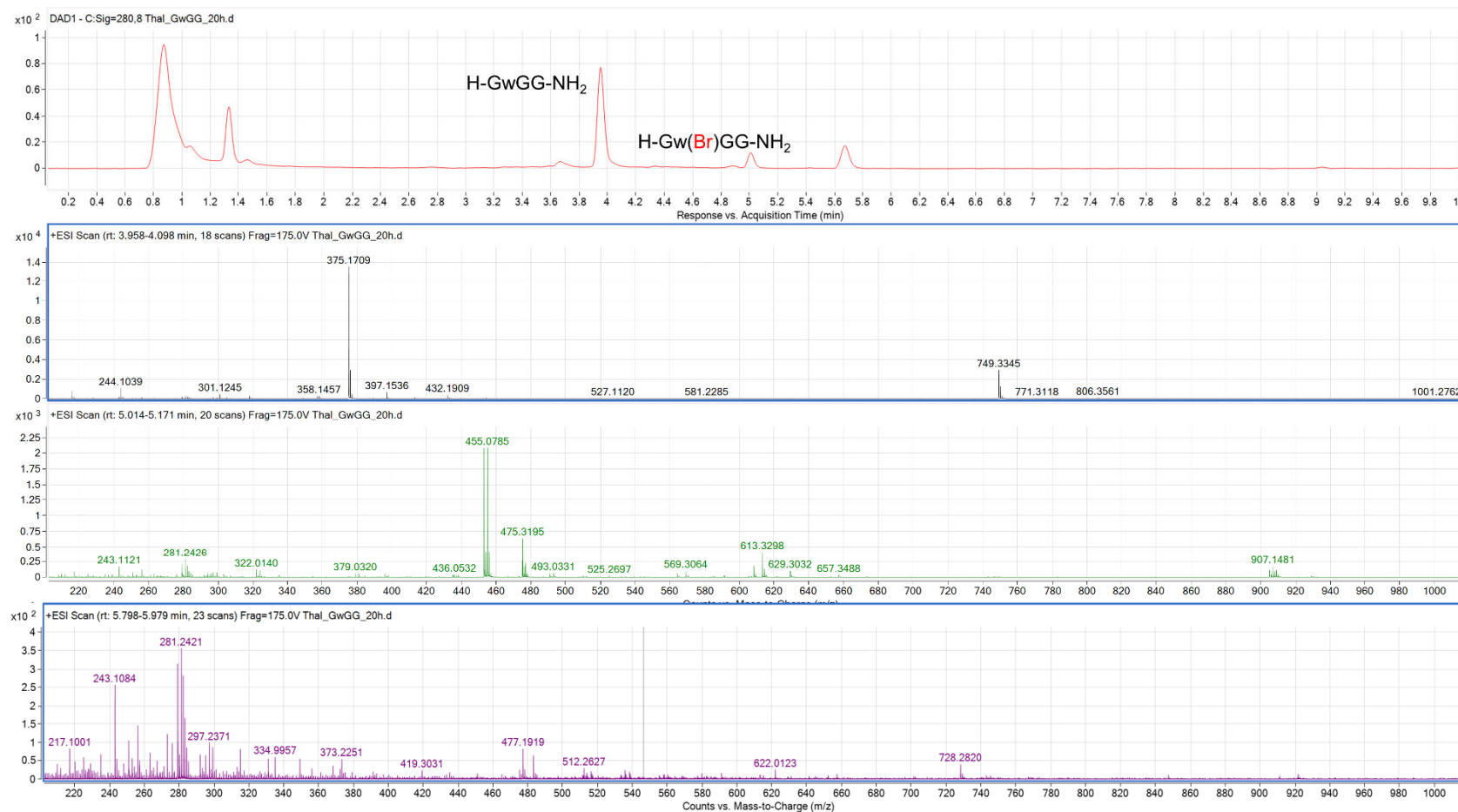
Figure S5. Impact of the position of tryptophan on bromination. HPLC-UV and -MS spectra after incubating peptide G-GwGG-NH 2 with Thal (20 h, 25°C) are shown. Positioning Trp in position 2 of the substrate peptide only gave bromination in a conversion of <5% corroborating the preference for peptides carrying an N-terminal Trp residue. H-GwGG-NH 2 m/z 375.17 (found); 375.18 (calc.) / H-Gw(Br)GG-NH 2 m/z 453.09 (calc.); 453.08 (found).
