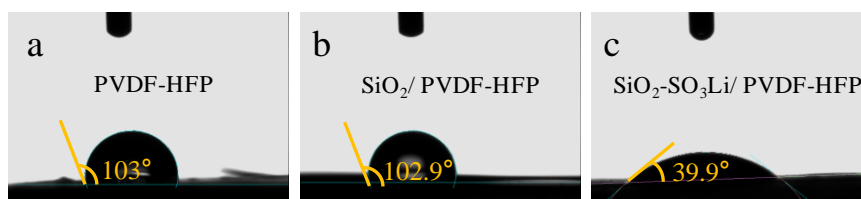
Supplementary Fig. 8. Contact angle between polymer film and liquid electrolyte (1 M LiTFSI/TEGDME): a PVDF-HFP; b SiO 2 /PVDF-HFP; c SiO 2 -SO 3 Li/PVDF-HFP.
