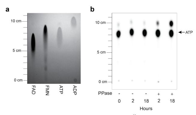
Supporting Figure S3: Attempted FADS enzymatic synthesis of <sup>32</sup>P-FAD resulted in aberrant <sup>32</sup>P product with PPase inclusion.
