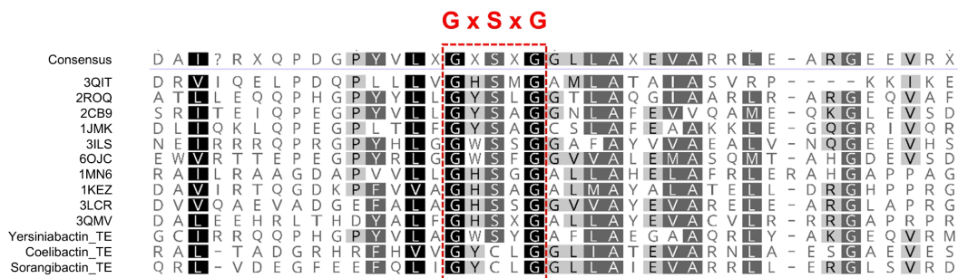
Figure S7 Alignment of TE domains. The sorangibactin TE domain is aligned with coelibactin TE, yersiniabactin TE and 10 structure available TEs from PDB database. The catalytic motif (normally GxSxG) is indicated in red dashed box.
