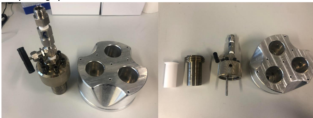
Figure S1. Small-scale autoclave setup. Left picture, the assembled Parr® autoclave and the on-site made heating block. Right picture, a PTFE inlay (30 mL max.), the disassembled autoclave and the heating block.
