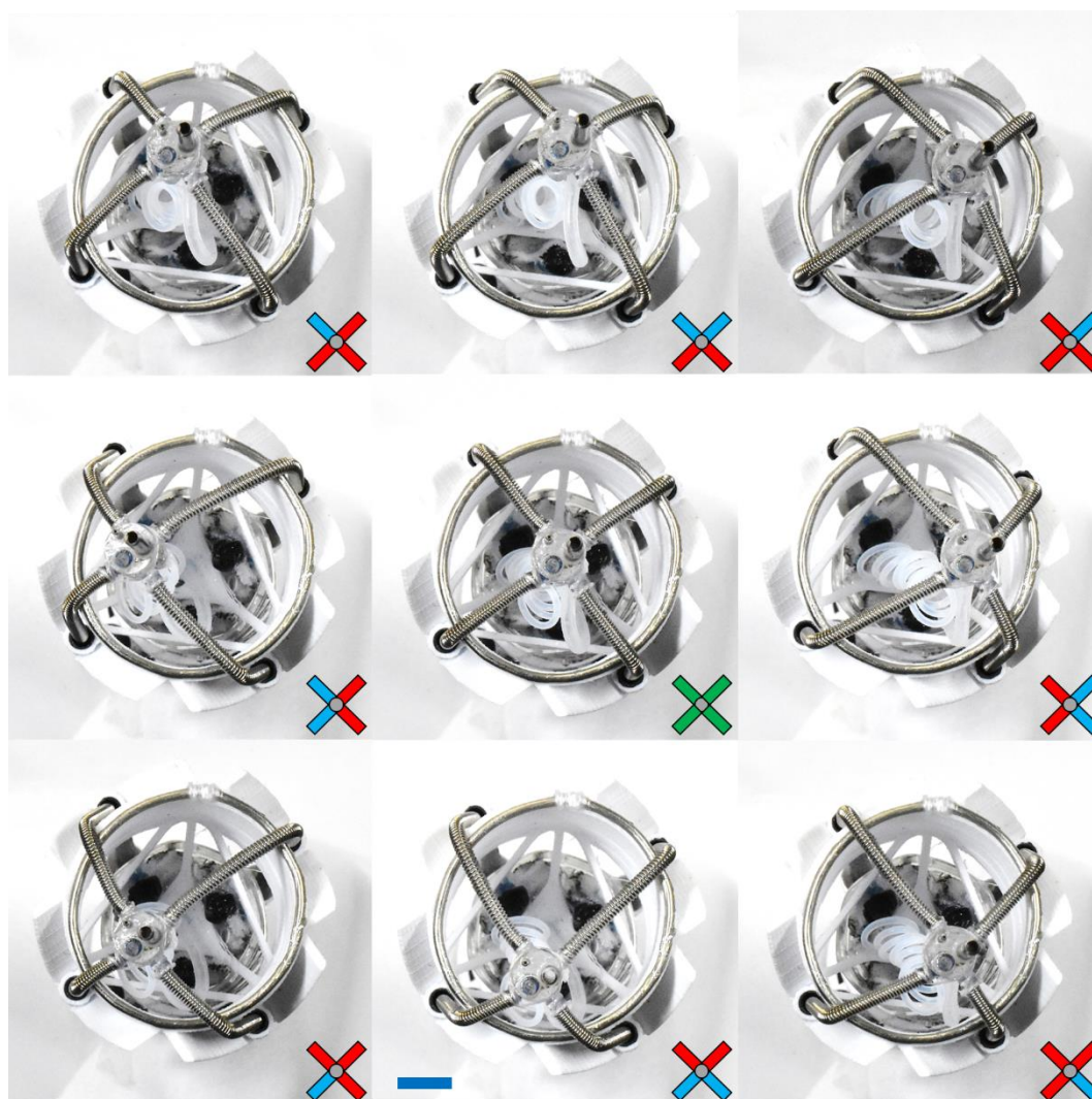
Figure S8. Various positions of the printing head with lengths of four SMAMs. In the bottom-right of each image, the pressurized muscles, the depressurized muscles, and the muscles in their initial state are shown in red, blue, and green respectively. Scale bar: 4 mm.
