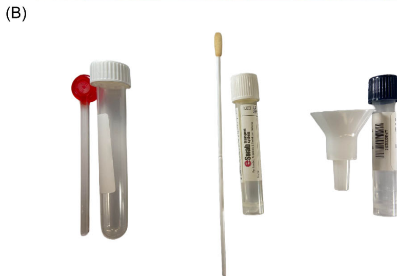
Figure S4. At-home saliva sampling devices for human subjects study. Self-saliva collection methods enable at-home sampling then shipping back to lab analysis. Three different collection methods included six CandyCollect devices, six ESwab™, and two Specimax Stabilized Saliva Collection Kits (from left to right). (A) wrapped (B) unwrapped.
