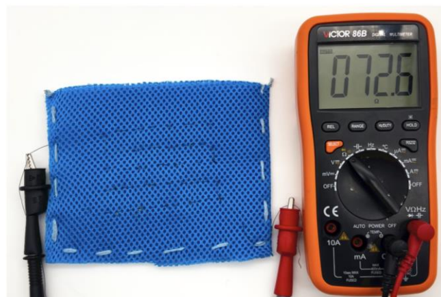
Figure S8. The internal resistance of the \text{Ag}_2\text{Te}_{0.6}\text{S}_{0.4}/\text{Cu} TE textile.
