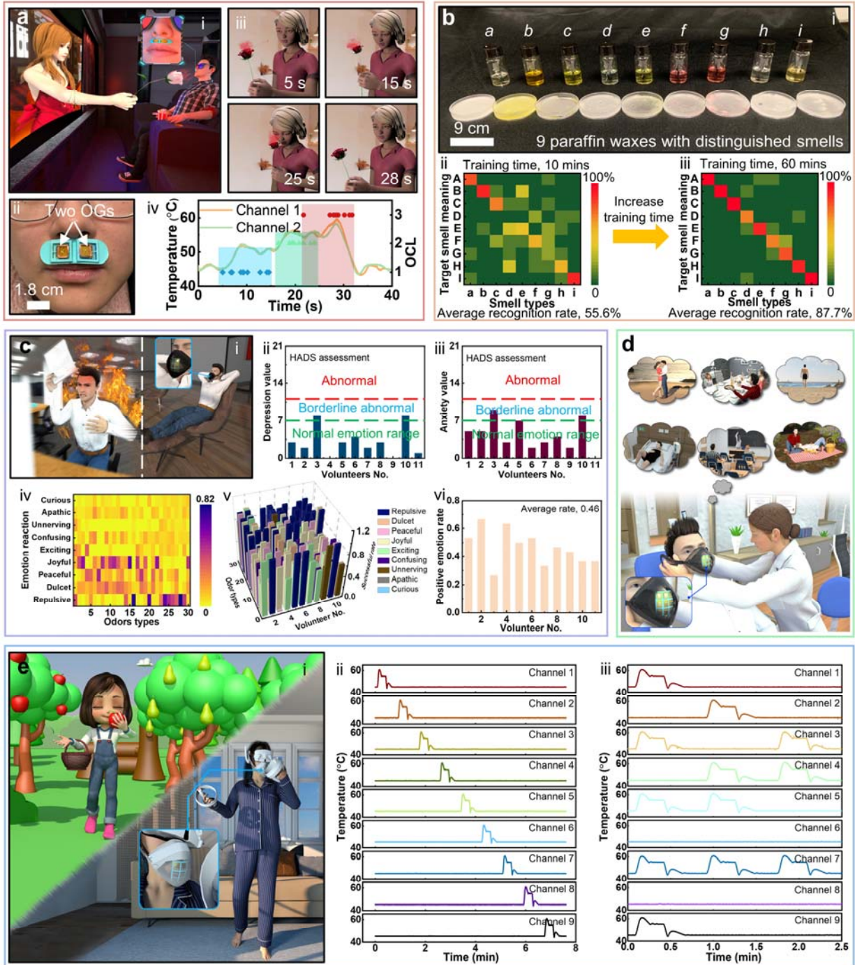
Fig. 4. Demonstrations of the olfaction interfaces. a A demonstration of the skin-integrated Device 1 in displaying olfaction feedback for providing an immersive experience to users during movie watching. Here, a girl in the movie is smelling a rose with the decreasing distance between the flower and her while the watcher could smell a more and more intense rose odor by wearing the olfaction interface. Here, OCL demonstrates the odor concentration level ranging from 1 to 3, corresponding to the low, middle, and high levels (iv). b A demonstration of the face-mask based olfaction interface in providing an alternative communication method, smell messages, for the disabled without the capability of vision and audio. By training users to link odors to specific information, the disabled users could efficiently communicate with others. c A demonstration of the Device 2 in assisting users to control their emotions as some
