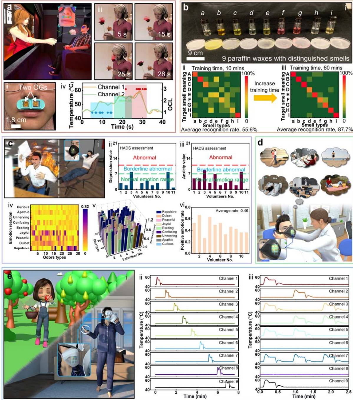
Fig. 4. Demonstrations of the olfactory interfaces. a A demonstration of the skin-integrated Device 1 in displaying olfaction feedback for providing an immersive experience to users during movie watching. Here, a girl in the movie is smelling a rose with the decreasing distance between the flower and her while the watcher could smell a more and more intense rose odor by wearing the olfaction interface. Here, OCL demonstrates the odor concentration level ranging from 1 to 3, corresponding to the low, middle, and high levels (iv). b A demonstration of the face-mask based olfaction interface in providing an alternative communication method, smell messages, for the disabled without the capability of vision and audio. By training users to link odors to specific information, the disabled users could efficiently communicate with others. c A demonstration of the Device 2 in assisting users to control their emotions as some specific odors could recall different human emotions. Here, all volunteers involved in the
