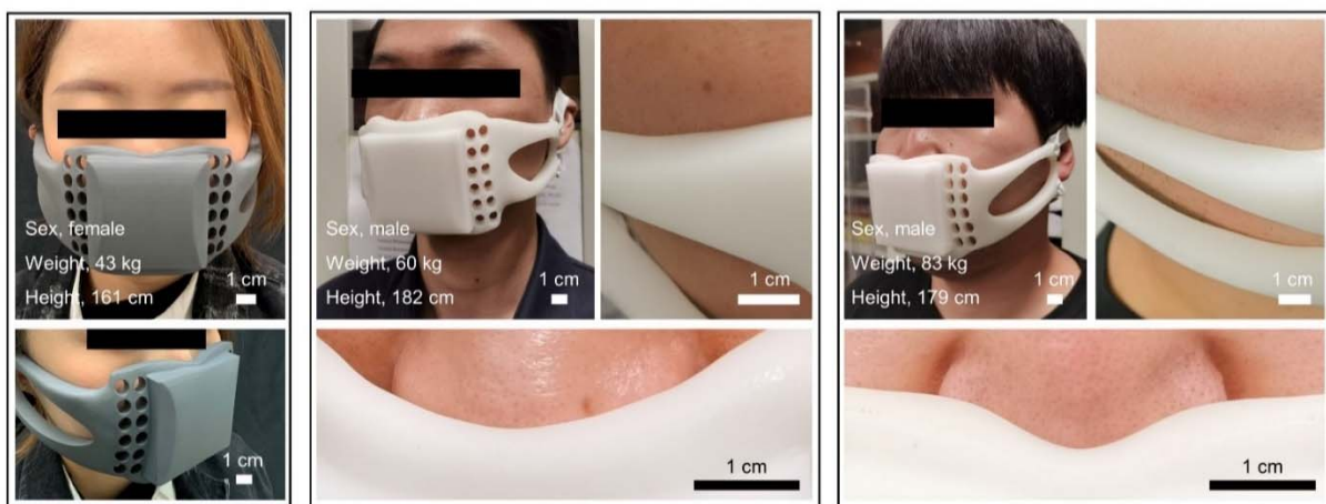
Fig. S7. Optical images of users wearing the Device 2, whose basic physical information have been provided. The flexible face mask substrate enables the wide applications for various users.
