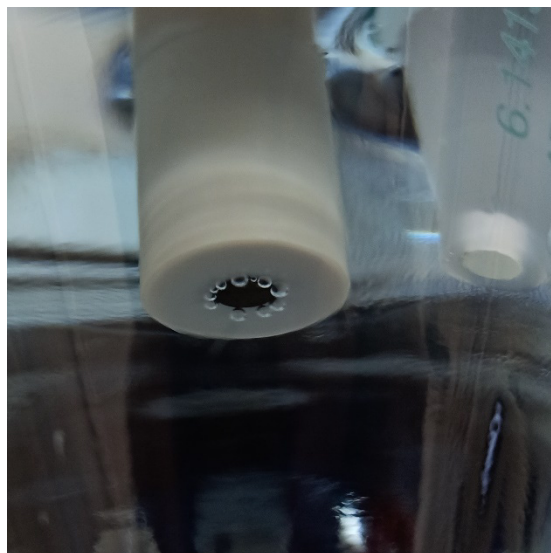
Figure S32. Evolution of O 2 bubbles during 100 CV cycles.
