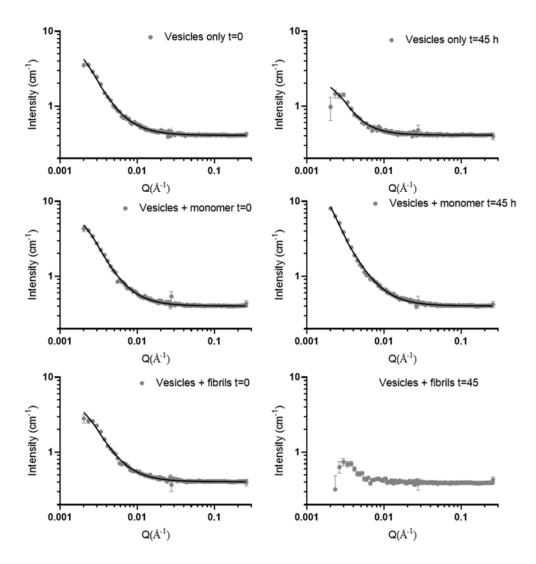
Supplementary Figure 5. Model fits to the SANS data at time 0 hrs and 45 hrs using the Guinier-Porod model. SANS data for SV in 42% D2O with aSyn monomer or fibrils is shown by grey spots. The Guinier-Porod fitting is shown by the black line, apart from for SV + fibrils t=45 where a good fit could not be achieved. Error bars represent s.d.
