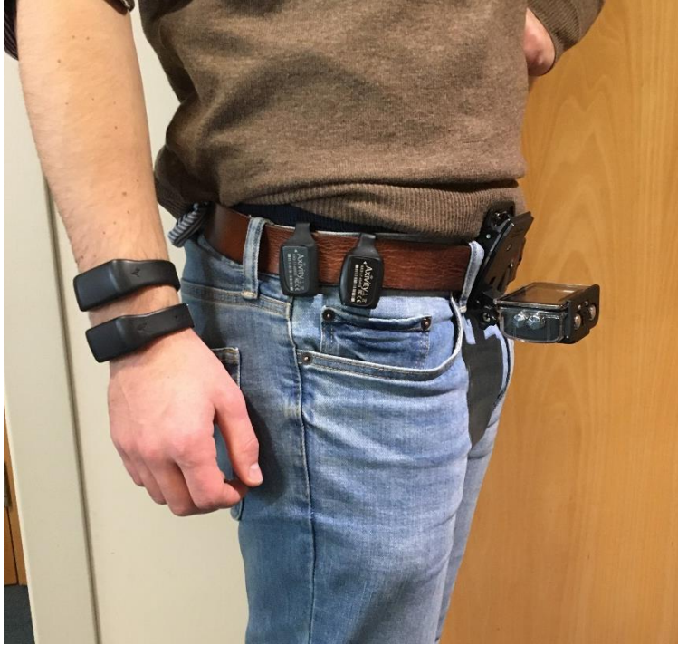
Supplemental Figure 1: A foot-facing action camera clipped at the participant's waistline recording video for step count annotation. The participant is also wearing Axivity AX3 accelerometers at the dominant wrist and at the hip.
