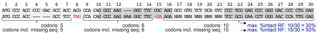
Fig. S13: Illustration of the computation of the maximum percent intact reading frame of a transcript.
