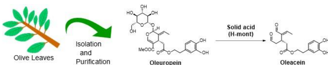
Figure S1. Oleacein synthesis from olive leaves.
