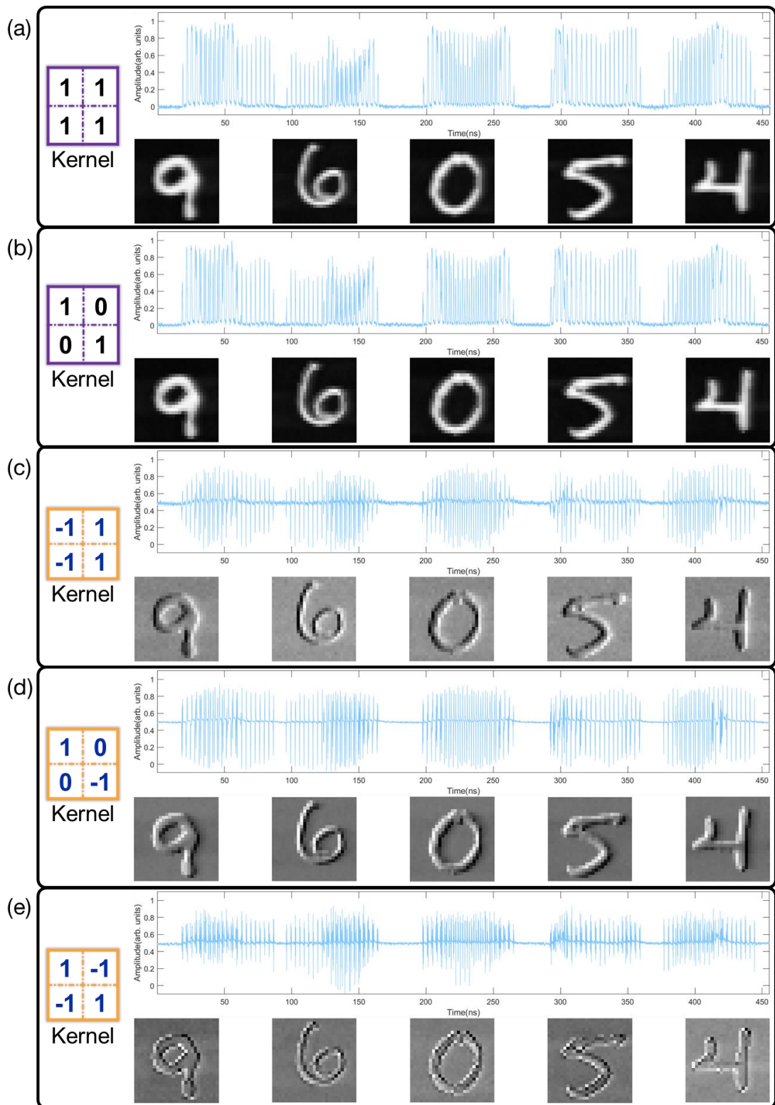
Supplementary Fig. 4 The temporal waveform obtained with the OCPU when performing the convolution operation with five kernels (corresponding to (a-e) respectively).
