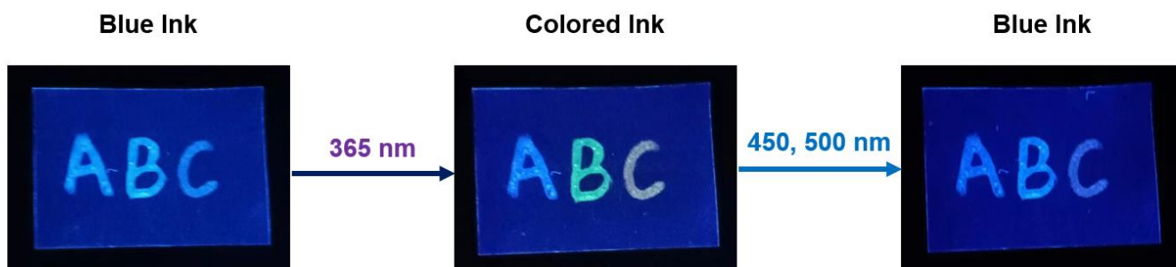
Supplementary Fig. 47 Fluorescent images of colored letters by direct ink writing at different states.
