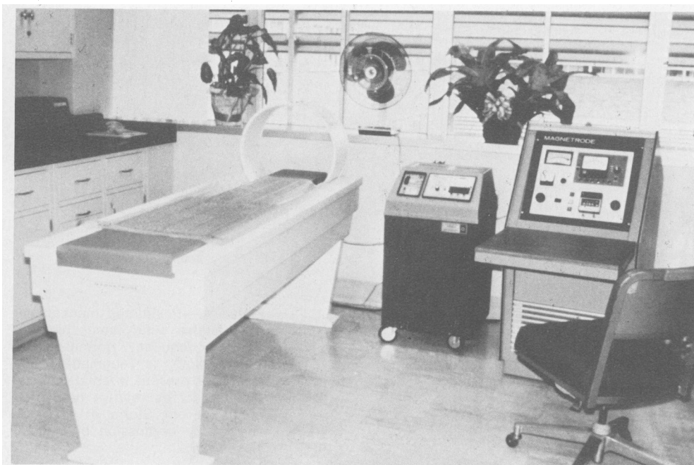
Figure 2. —Circular magnetic-loop induction applicator (20-inch trans-thoracic and transabdominal electrode shown).
