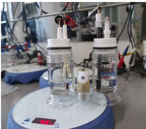
Supplementary Figure 4. Reaction setup for the electrochemical synthesis of cyclohexanone oxime over a Cu-S cathode.
