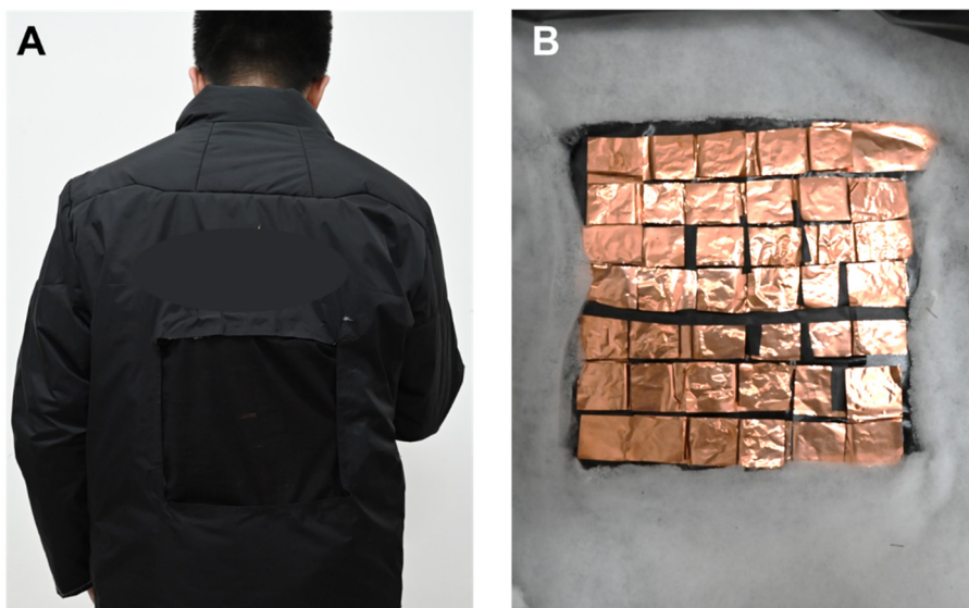
Fig. S15. A , Thermolectric jacket. B , The padded network-based FTEG.
