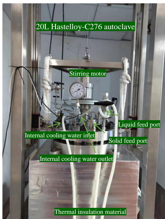
Supplementary Figure 2 Mechanical stirring autoclave for the acetolysis of PET.
