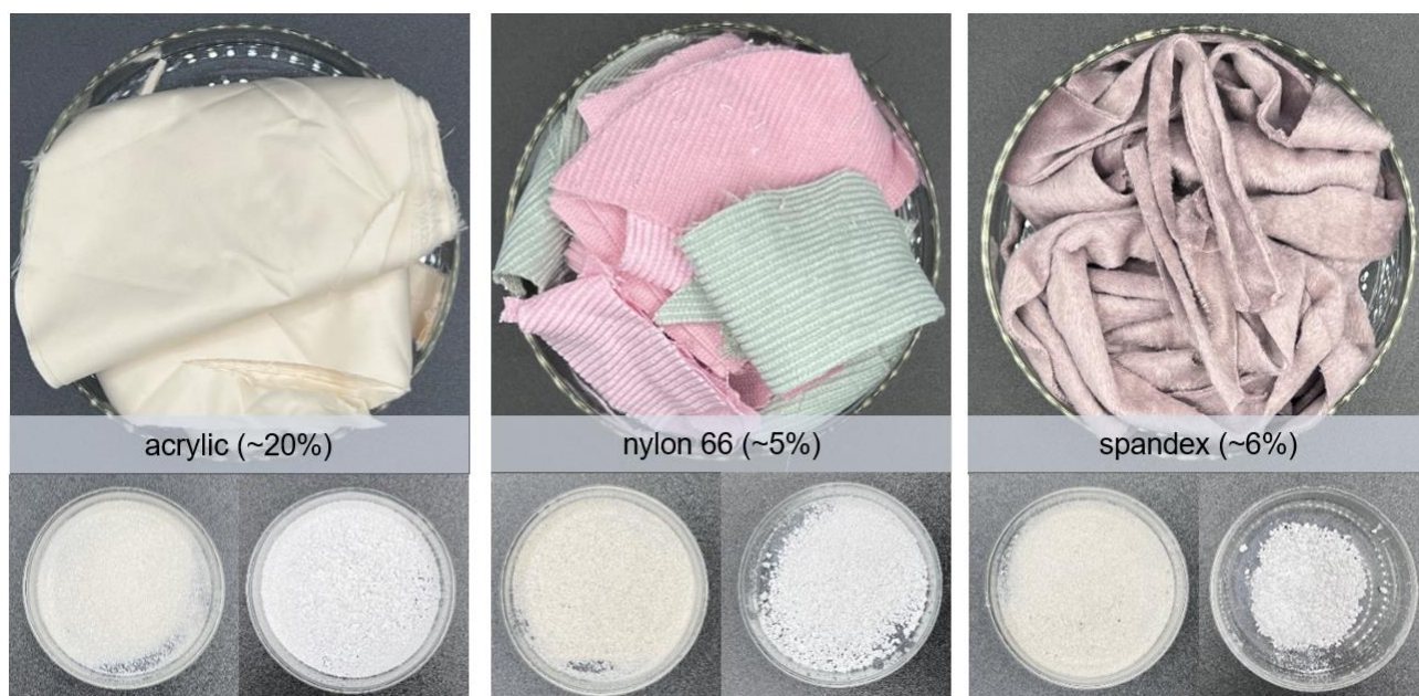
Supplementary Figure 12 Acetolysis of various textiles blended with PET. Decolorized terephthalic acid obtained from different textiles yields greater than 90% and purity over 99.7% by decolorized method 1. Satisfactory results of acetolysis are due to the excellent dissolution/decomposition effect of acetic acid on most impurities.
