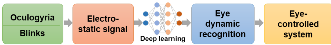
Supplementary Fig. 1. Overview process of the eye-controlled input modality for human-computer interaction.
